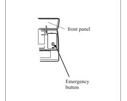
The emergency button is located on E-box cover of the unit under the front panel.
