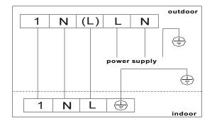
Note: For some models the wires has been connected to the main PCB of indoor unit by manufacturer without terminal block.
