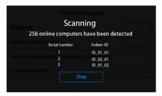
After the scanning is completed or manually stopped, a pop-up box will appear to confirm with the user whether to save the scanning results. After confirmation, the scanning information will be written to the system.
