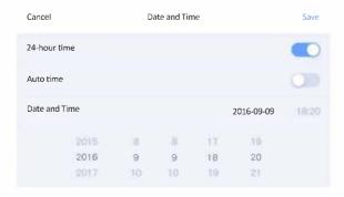
After the function of automatic time checking is enabled, the system will connect to the time checking server of external network to automatically check the time. The user cannot manually set the date and time at this time.
