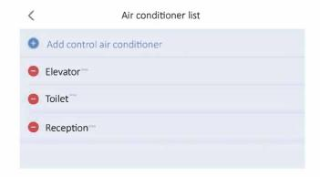
Click "Add Air Conditioners Controlled" to enter the unit selection interface. The list of units that can be added is displayed in the unit selection interface. When selecting units, the user can switch to the mode of selection by group or selection by unit, and multiple items in the list can be selected. Among them, the units displayed in gray have been added.
